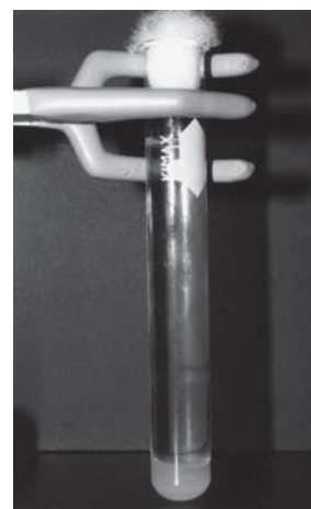
Figure 2 Gradient tube culture with cotton or synthetic wool plug, water sample, and agar nutrient source.
