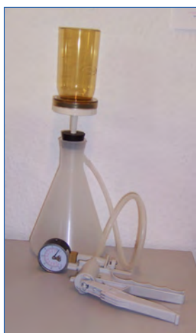
Figure 5. Filtration equipment and hand pump.
