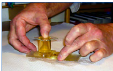
Figure 9. Replacing the sedimentation chimney with a cover glass.
