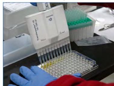
Figure 11. After microplate is read at 650nm, row "A" is acidified with 50 µL of 10% H 2 SO 4 ; optical density is recorded at 450 nm for row "A". The measure at 650 nm is considered low sensitivity while that at 450 nm is considered high sensitivity. For positive samples, the optical density at 450 nm should be roughly 2X that at 650 nm.
