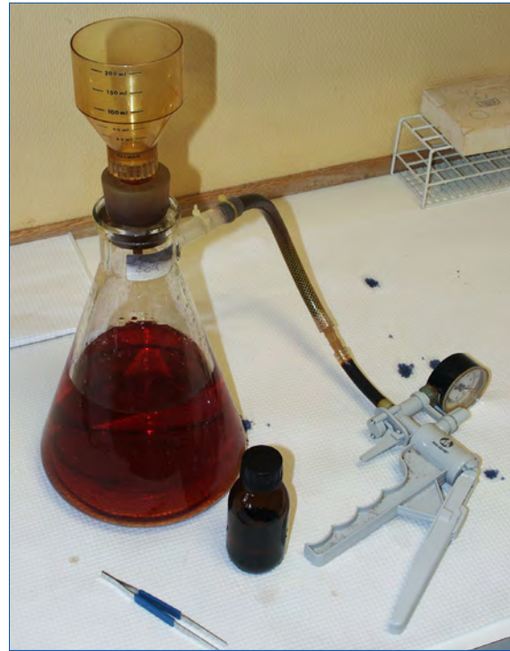
Figure 1. Filtration manifold and hand held vacuum pump.
