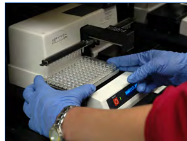
Figure 8. Microplate being placed on processor after prongs added to processor arm.
