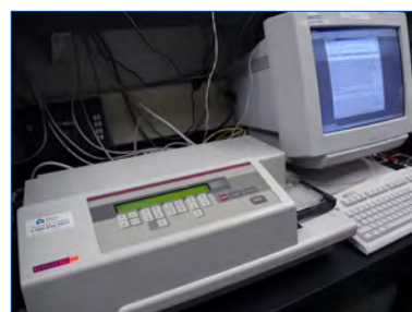
Figure 10. Microplate is placed on microplate reader cradle; optical density is recorded at 650nm for row "A" (wells in which colour development has occurred).
