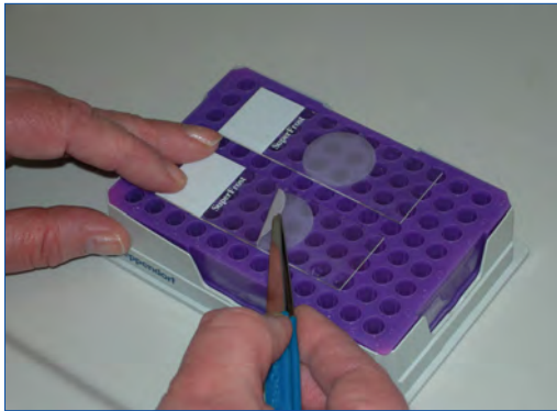
Figure 2. Removal of filter from microscope slide using forceps.
