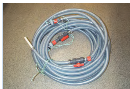
Figure 6. Tube for integrated water sampling.
