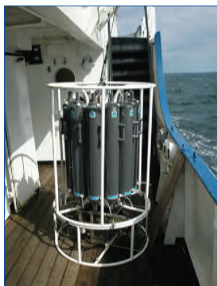
Figure 4. CTD with rosette and Niskin-type water bottles. An in situ chlorophyll a fluorometer is also mounted.
