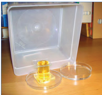
Figure 8. Sedimentation, with a Petri dish filled with water. A plastic box covers the sedimentation chamber and the Petri dish to maintain the humidity.
