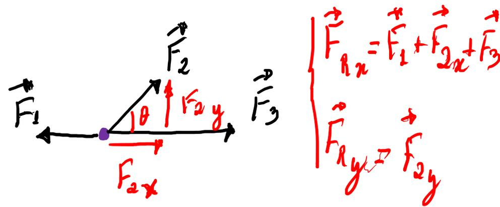
$$F_{Rx} = -6,0 + 12 \cdot \cos 45^\circ + 14 \quad \left\{ \begin{array}{l} F_{2x} = F_2 \cdot \cos \theta \\ F_{2x} = 12 \cdot \cos 45^\circ \end{array} \right.$$
